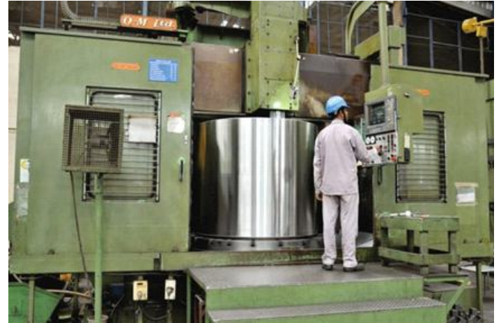
Centrifugal Basket Machining on VTL
