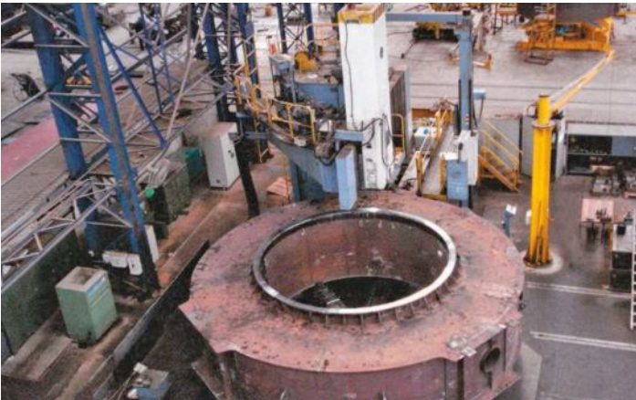
Sub Structure on Russian CNC VTL
