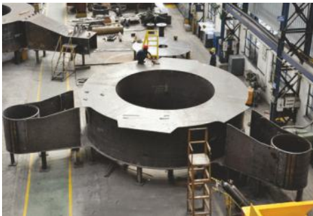
Stacker Reclaimer - Sub Structure
