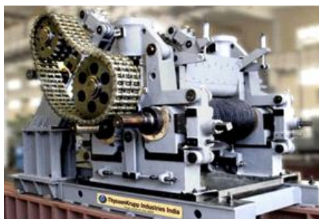
Mill Assembly with Toothed Roller Pressure Feeder
