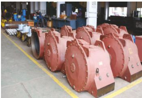
Roller Station Bearing Assembly
