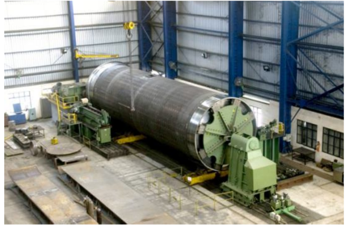
Mill Shell Machining on Lathe
