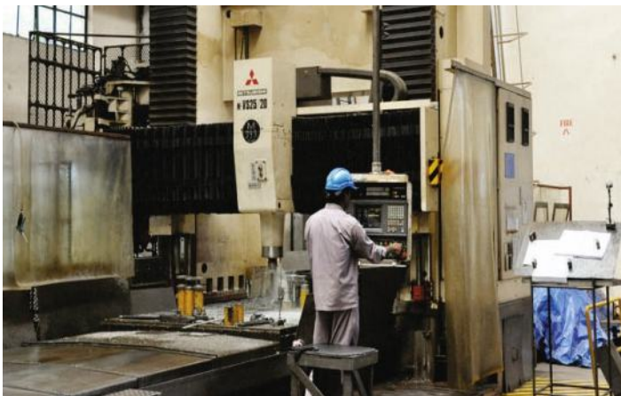
End Shield Toothed Ring Machining on Plano Miller
