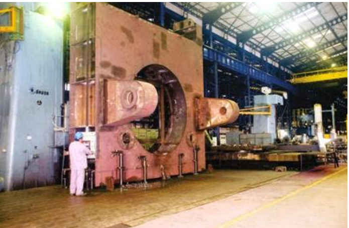
Slew Platform Machining on Skoda
