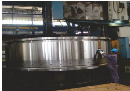
Mill Tyre Under Machining in Russian VTL
