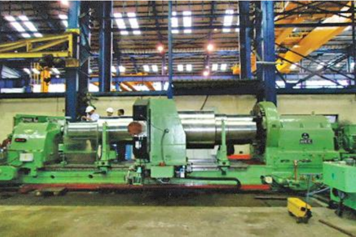
Polycom Roller Shaft Under Machining
