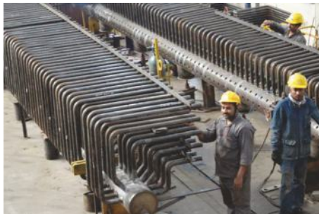
Waste Heat Recovery Boiler with Bend Tubes
