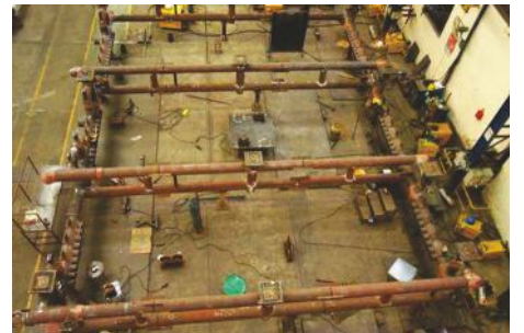
Waste Heat Recovery Boiler Header Frame
