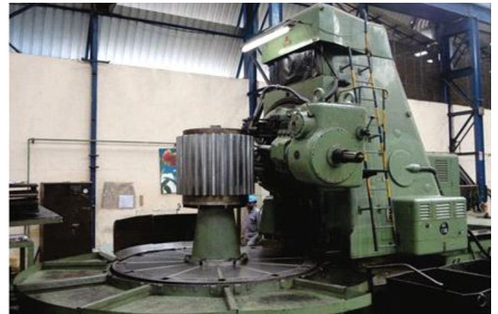
Pinion Machining on Hobbing Machine
