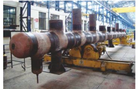
Common Steam Distribution Header
